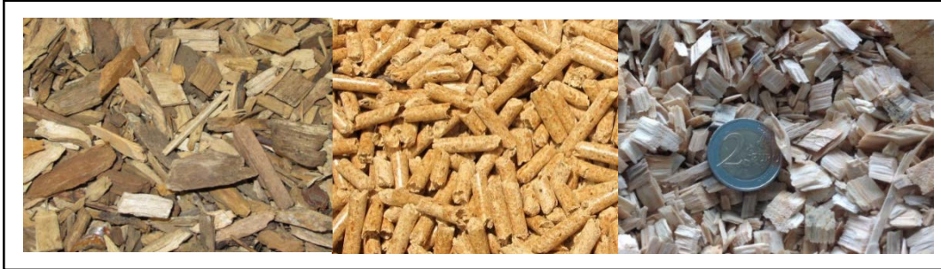
Figure 1: Fuels investigated wood chips, wood pellets, DMC Fuel™ (from left to right)
